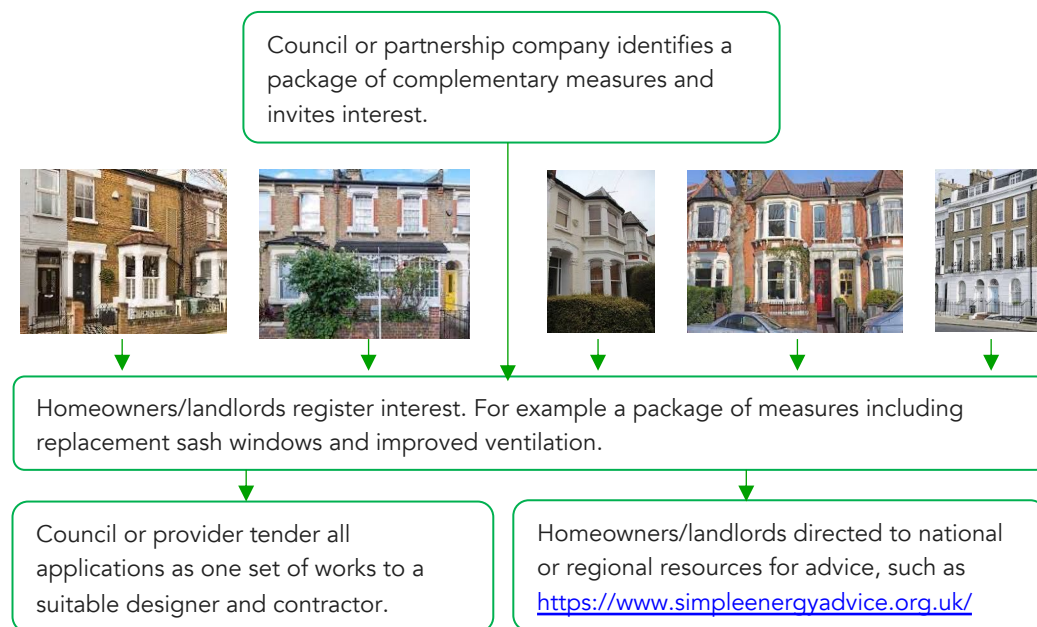
Example outline process for aggregating a package of works across multiple homes
